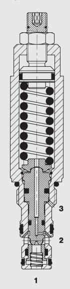
The counterbalance valve RS08 is a direct-acting poppet valve. Its function is to control the speed of a consumer according to the inlet flow. It also prevents the consumer from overrunning if there are retracting loads and ensures smooth action in consumers. In loadholding applications, it can be used as a hose-break valve.
