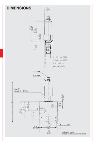
To raise a load, flow is permitted from pump port 2 to consumer port 1 via the built-in check valve.
